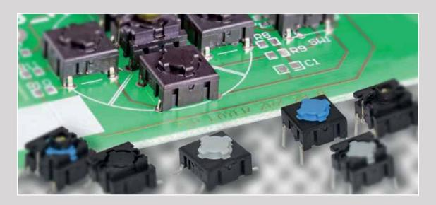
multimec® 5 series is the new generation of 3A, 3F, 4A and 4F switch. In principle the multimec® 5 series is very similar to the 3 series - it has the same pin layout, the same dimensions and the same electrical specifications.
